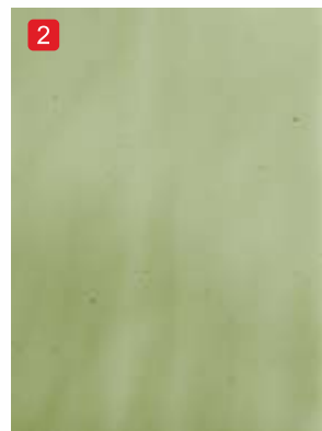
Fig. 2 Film after the application of PFAS FREE PPA additive
